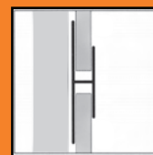
PVC H JOINT/DECOR STRIP To make a H joining of panel edges or as silver and white decor strips White (GET8HTWH) Silver (GET8HTSI)
