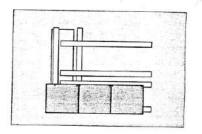
2. Second under eaves course. Use a slate and a half width to the verge. Before fixing it should be drilled as illustrated. This allows for fixing of a copper disc rivet to the first full-size course.
