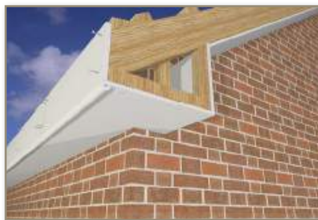
Fig 3. Standard fascia installation illustration showing typical fixing of fascia components.
